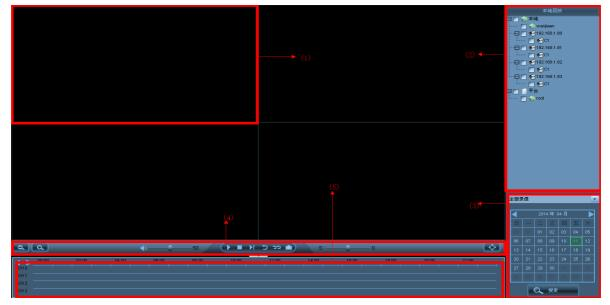
Local Playback: it is the function module of playback of video recording files. It supports 4 chplayback at the same time in maximum. It can search the recording video files by date and also check the specific time by timeline. The recording video file format is H.264.
