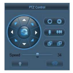
[1] Direction control button, can control eight direction respectively: up, down, left, right, right-up, right-down, left-up, left-down and middle button for automatic scanning;
